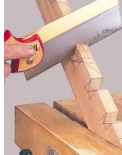
To reduce the wear on your cutters, saw out the waste from areas such as the scoring arches.
