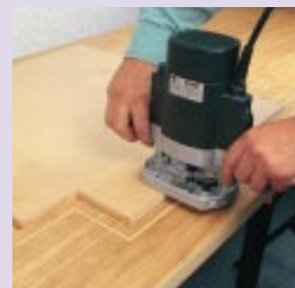
Internal and external templates are used when repeating inlay recess patterns on a number of similar patterns.
