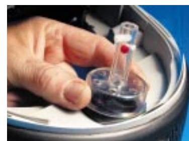
An airflow indicator is supplied to allow testing of the airflow to ensure that the respirator meets the minimum airflow requirement of 140 litres per minute.
