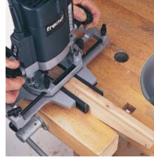
For safety and accuracy, it is advisable to cut the inclined ramp grooves of the Marble Run on a router table. If using the router handheld, fit a second side-fence to keep the groove centred.
