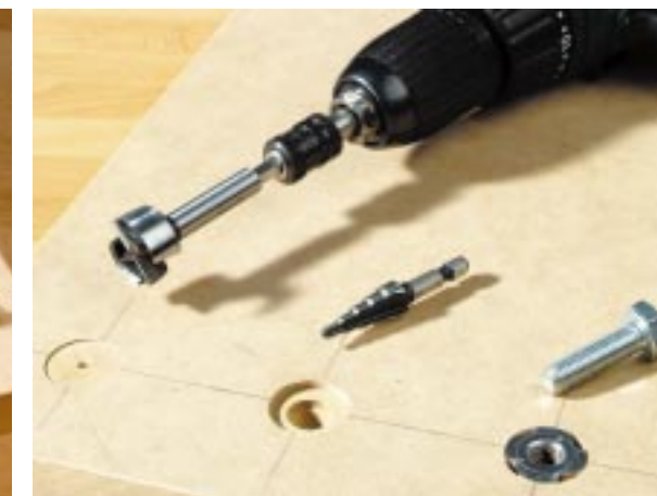
A combination of boring and drilling bits ensure that fittings are fitted neatly and securely.
