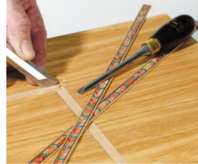
Use a sharp chisel to remove the rounded corner left by the router cutter, taking care not to widen the recess.
