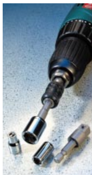
Square drive adaptors allow 1/4 and 3/8 inch hex drive sockets to be used in a cordless drill.
